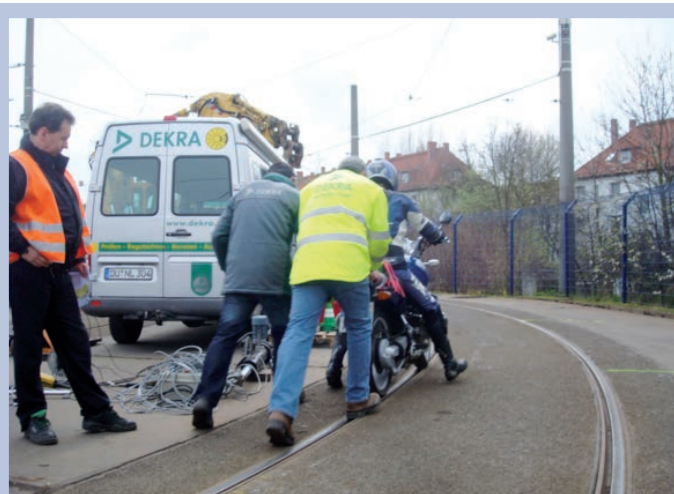
Fig. 3: Test ride of a motorbike along the conditioned curved track
