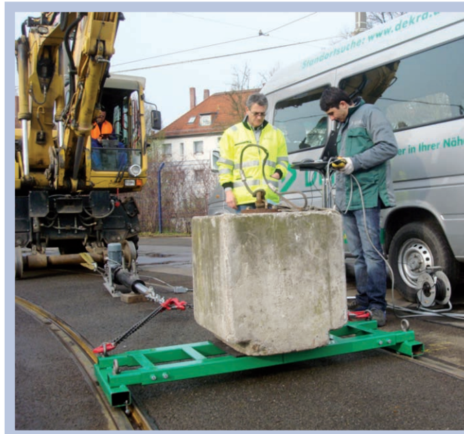
Fig. 2: Measurements of the friction coefficient (parts of rubber tyres were used as the friction partner on the rail head)
