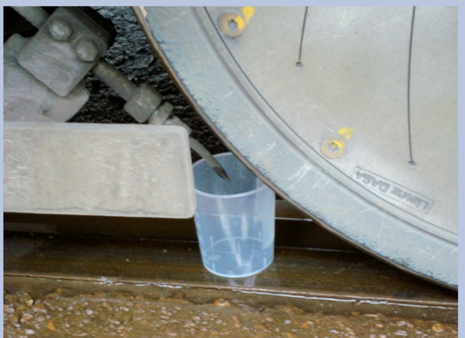
Fig. 1: Measuring the quantities sprayed onto the rail head
