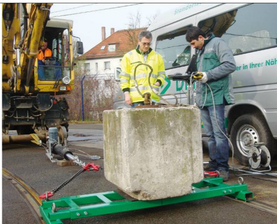
Coefficient of friction measurements (rubber tyre sections were used as friction bodies on the railhead)
